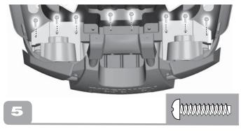
• Now, fit eight more #8 x 3/4" screws into the remaining holes in the front end and tighten them.
